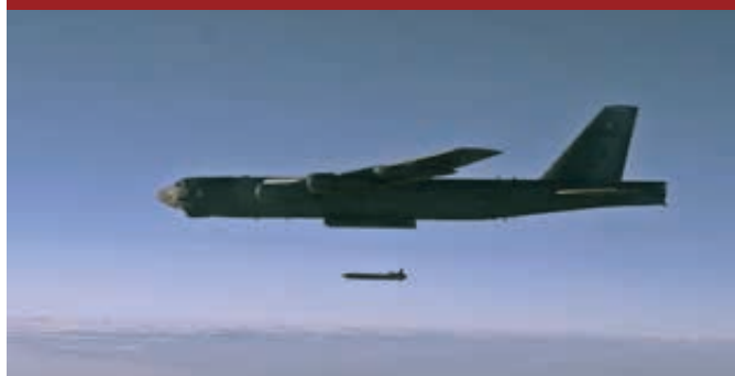
AGM-86B Air-Launched Cruise Missile dropped from a B-52H Stratofortress, Utah, 2014 (U.S. Air Force photo/Staff Sgt. Roidan Carlson)
